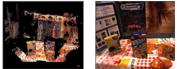
Fig. 10 Captured range data from a stereo camera
