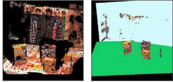
(a) a 3D point cloud (b) planes extracted
