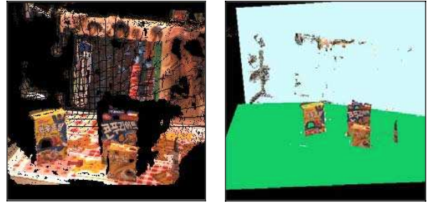
(a) a 3D point cloud (b) planes extracted Fig. 3 The scene with planes extracted.
