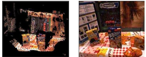
Fig. 10 Captured range data from a stereo camera
