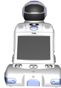
Fig. 3 iRobi: a home robot for education and security, used for implementation of CRE [the courtesy of Yujin Robotics Co Ltd.]
