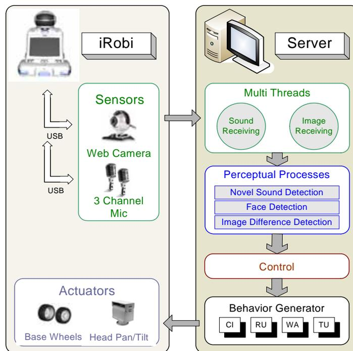
**Fig. 4.** The design of robot security system.
