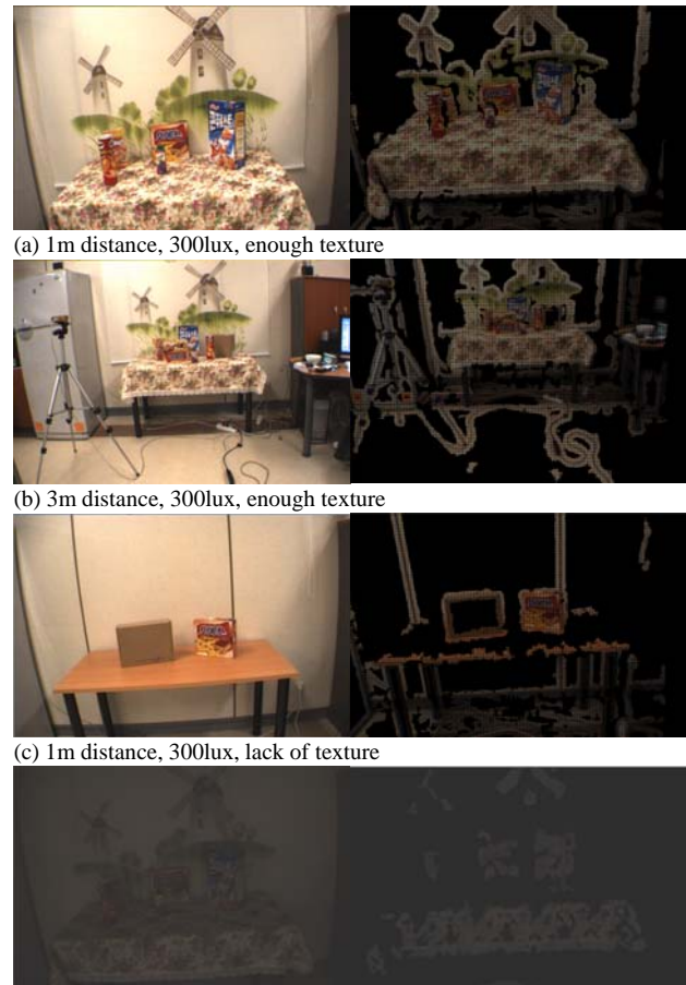
(a) 1m distance, 300lux, enough texture (b) 3m distance, 300lux, enough texture (c) 1m distance, 300lux, lack of texture (d) 1m distance, 50lux, enough texture Fig. 1. 2D image and 3D point cloud captured by a single stereo camera in various environmental conditions.
