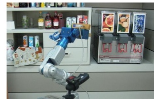
Figure 3: A home service robot with a stereo camera system searching for a juice dispenser object in a kitchen.
