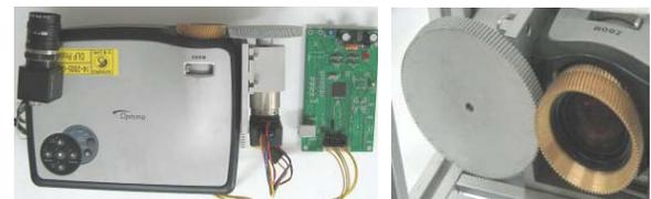
Figure 7. Diagram of projector-camera system (top), implemented system (bottom left) and gear module (bottom right).
