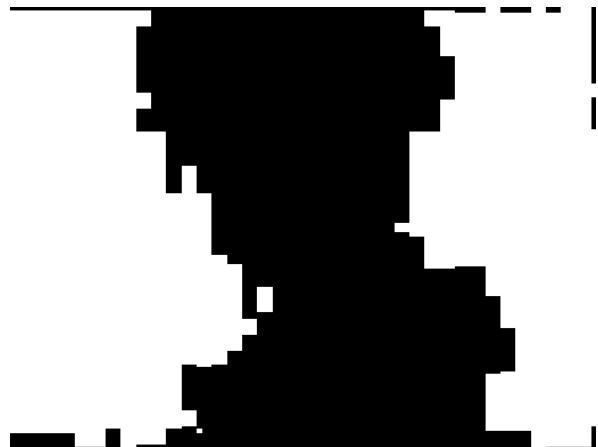
Figure 14. Segmented blur-map, the board's area is obtained (white colour is 1, black colour is 0).
