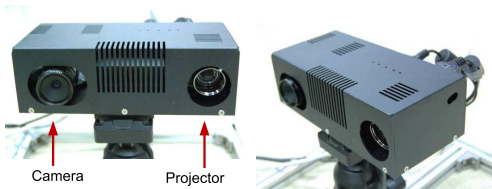
Fig. 9: The setup of the structured light system (Pico system).
