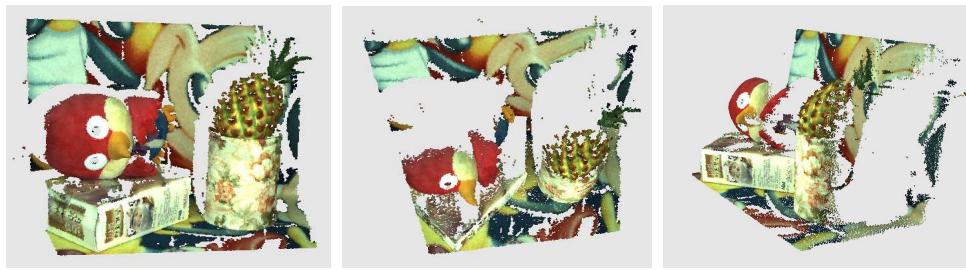
Fig. 12: The 3D point cloud of the scene captured by Ray-Tracing codec (left: front view; center: top view; right: side view).
