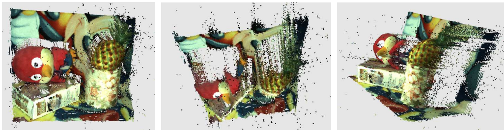
Fig. 13: The 3D point cloud of the scene captured by Gray code inverse (Trobina's method) (left: front view; center: top view; right: side view).
