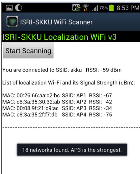
Figure 2. Android application that was developed and used in RSS data collection – only APs that are controlled by the experiment are displayed after filtering the non-related APs
