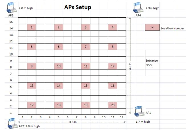
Figure 1. Setup Area of the Controlled Environment
