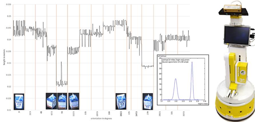
**Fig. 3.** Left: Example of singularity in height measurement of milk box in certain orientations causing feature likelihood to be multimodal. Right: 3rd generation of HomeMate cognitive consumer robot
